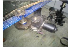
Figure 2.3 Spur Gear
