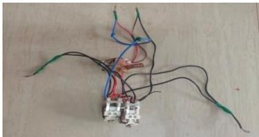
Figure 2.11 Remote Receiver with Relay Circuit
