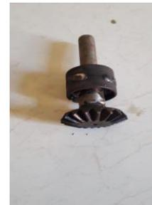
Figure 2.4 Bevel Gear
