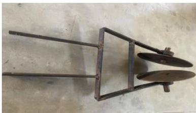
Figure 2.10 Disc Type Bed Former
