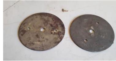
**Figure 2.7 Metering Disc**
